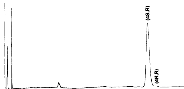
Fig. 2. HPLC chromatogram illustrating the limit of quantitation of the RS-93522-004 (4 R,R ) bis-camphanate diastereomer.
